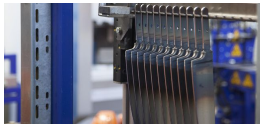
Following contour cutting, the blades wait for pins to be fitted and then go for grinding and hardening.
