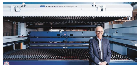
When combined with the LiftMaster Compact and Part Master, the system fully automates parts cutting on the refrigerator manufacturer's production
