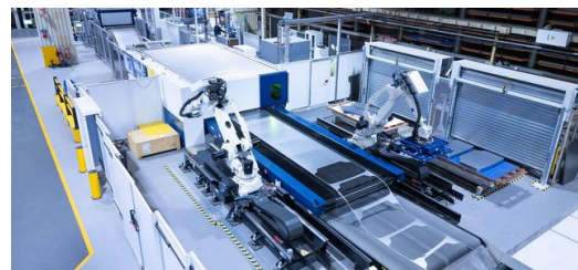
A general view of the TruLaser 8000 Coil Edition: This picture shows how much less sheet metal waste is left over when Fendt cuts from a coil instead of a sheet.
