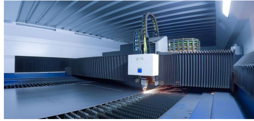
The laser head whizzes across the seemingly endless sheet metal strip and cuts the contours of the outer skin parts of the Fendt tractors.
