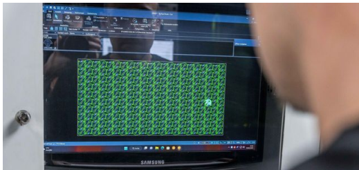
The CoolLine option guarantees consistent temperatures during laser cutting. "This means that we can nest parts much more closely and save material," Denis Lozusic is pleased.
