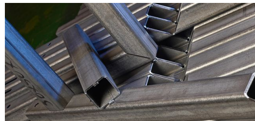
The technology package for bevel cuts provides high-quality 45° cuts. The great cutting speed also makes this highly productive. Picture: Escherich Fotografie
