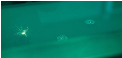
<p>Aesculap utilises lasers for various applications, including the additive manufacturing of acetabular cups.</p>
