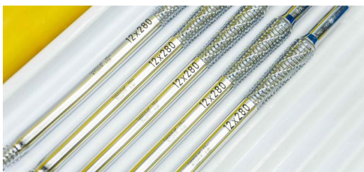
The company uses TRUMPF's TruMicro Mark ultrashort pulse lasers to apply robust and durable markings.
