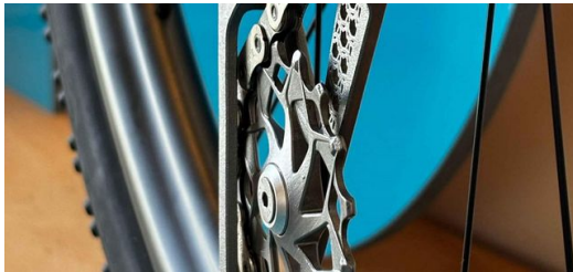
Titanium components: For the same bicycle, Dangerholm and the TRUMPF specialists at Faction Bike Studio used a TruPrint 1000 to 3D print exposed and vulnerable rear derailleur components using titanium.
