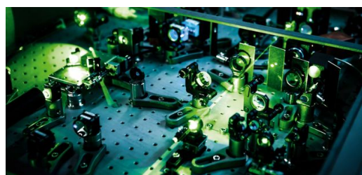
Her research team in Lund, Sweden, uses femtosecond laser pulses to generate high harmonics, which in turn are used to generate attosecond laser pulses which help us to observe atomic processes.
