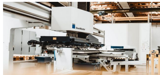
Automation: The SheetMaster supplies the TruPunch 5000 with the required material, thereby increasing efficiency and reducing employees' workload.
