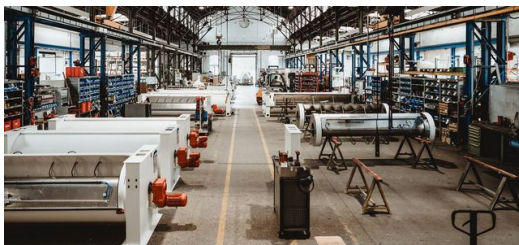
Core business: In its historic production hall, Cimbria Heid manufactures trieur machines for sorting seed and grain.
