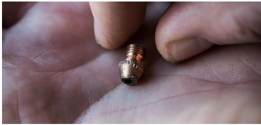
This cutting nozzle completed a record 273 shifts before being replaced. The damage was caused by a minor operational glitch at the machine. Picture: Thorsten Doerk
