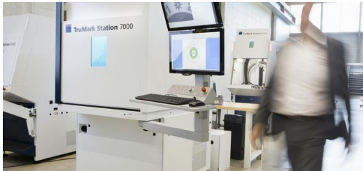
The edition engraving for the Meister S Chronoscope Platinum Edition 160 was created in a TruMark Station 7000 equipped with the new generation TruMicro Mark Series 2000 ultrashort pulse laser.
