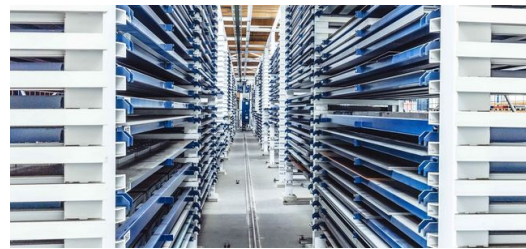
The fully automated STOPA store with 400 spaces is one of the highlights of the extensive automation measures from Tim Ungerer.
