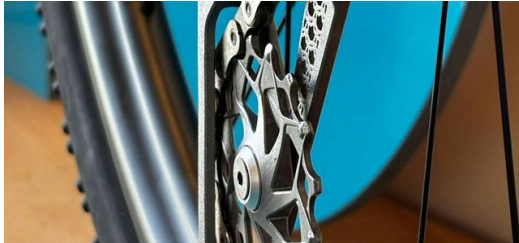
<p>Titanium components: For the same bike, Dangerholm and the TRUMPF specialists printed rear derailleur components on a TruPrint 1000 with titanium for Faction Bike Studio.</p>
