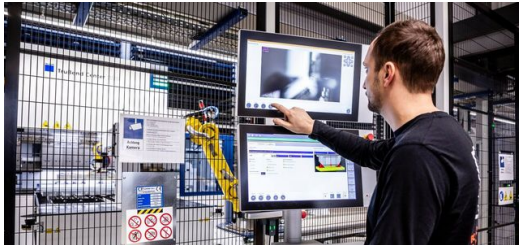
The TecZone Bend programming software in combination with SimulEasy ensures process reliability. This allows 3D simulations including collision monitoring to be generated before the bending process.
