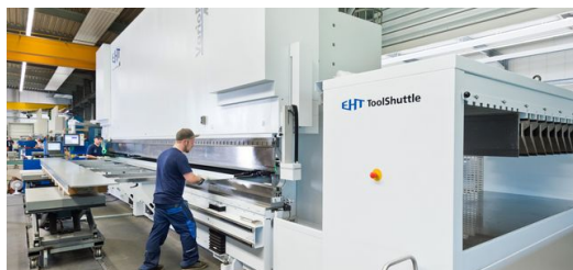
The ToolShuttle tool magazine connected to the VarioPress makes jobs easier and faster. The ToolShuttle contains the two bending dies that cover 99 percent of the bending jobs performed at Schrag. Picture: Dirk Egelkamp
