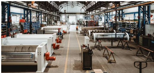
Core business: In the historic production hall, Cimbria Heid manufactures trieurs, machines for sorting seed and grain.
