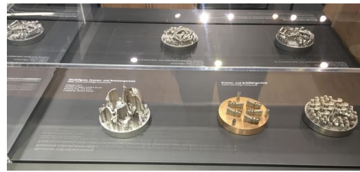
Substrate plates with 3D-printed dental prosthesis.
