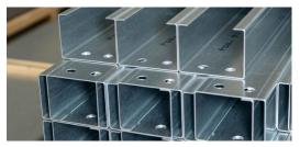
Precise product analyses by the SCHRAG project group show that some profiles exhibit a certain degree of standardization. In the future, these profiles will be produced automatically on a roll forming line at SCHRAG's Hamburg Seevetal site.
