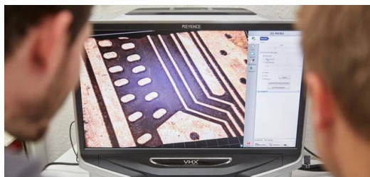
Part of the visual inspection involves documenting homogeneous ablation. The ablation zone is dark and shows the plastic surface. The key to successful machining is to ablate the gaps cleanly to provide electrical insulation between the conductive tracks. (Picture: Claus Langer)
