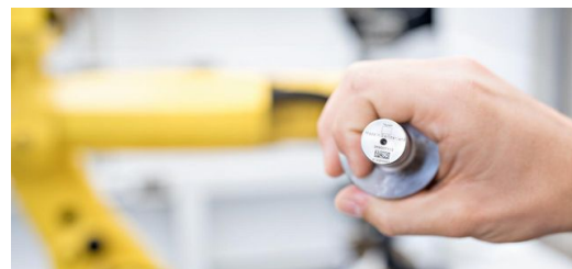
Customization: Each blank is uniquely identifiable through its data matrix code. Picture: Claus Morgenstern
