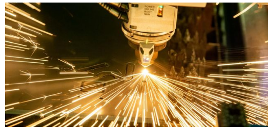
<p><span lang="EN-US">With EdgeLine Bevel technology, a TRUMPF standard machine for laser cutting produces beveled cutting edges on the contours of the component. </span></p> – TRUMPF / Martin Stollberg
