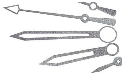
Cutting to specification with an ultrashort pulse laser: watch hands made of 0.05 millimeter thick stainless steel. The slotted recesses provide space for a subsequent application of fluorescent material. Picture: TRUMPF
