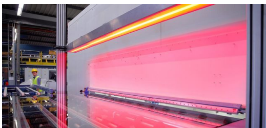
An ultrathin laser line — thinner than 100 micrometers — briefly heats the functional coating on sheets of glass to over 500 degrees. Image: Ralf Kreuels
