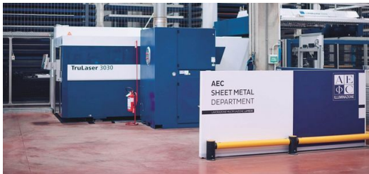
<p>The TruLaser 3030 fiber 2D laser-cutting machine laid the foundations of AEC Illuminazione’s close partnership with TRUMPF. Its connection to an automated storage system made production much faster.</p>
