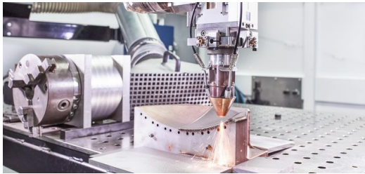
Time to process the order – a TRUMPF laser applies a metal layer onto a tool for a press in the automotive industry.
