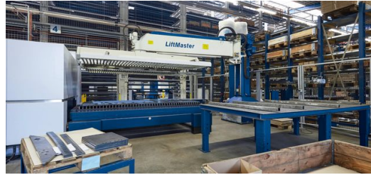
A Stopa storage system takes care of supplying materials while a LiftMaster makes it easier to handle parts. (Picture: Claus Langer)
