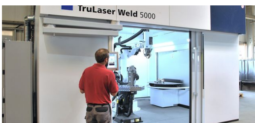
Significant savings: sheet metal fabricator Schink operates its TruLaser Weld 5000 laser welding cell and TruLaser 3040 laser cutting machine in what's known as a laser network. That means the two systems share a 4-kilowatt TruDisk 4001 solid-state laser source. Image: Peter Klingauf
