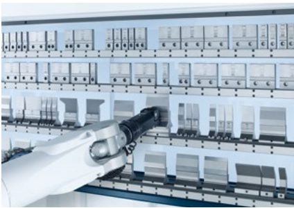
The ToolMaster Bend equips tools fully automatically.
