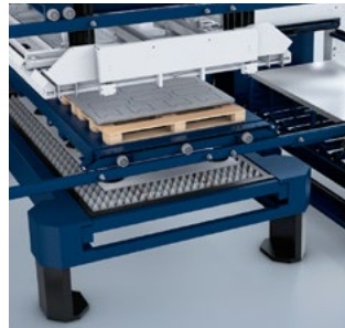
The synchronous loader loads and unloads in parallel, thus increasing productivity.
