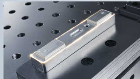
Welding a battery can cap, material: aluminum
