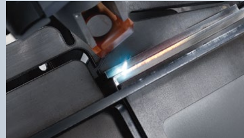
Welding of a battery tray, material: aluminum 6000
