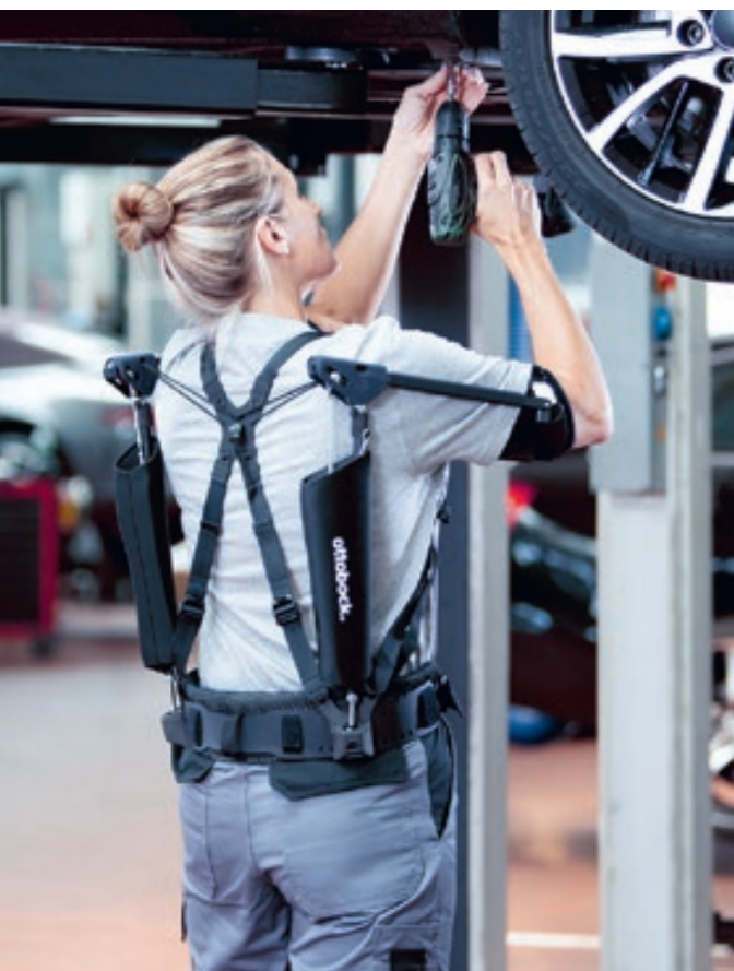
Making work easier: The Paexo Shoulder exoskeleton transfers the weight of the user's raised arms to the hips, providing relief for the muscles and joints in the shoulder area.
