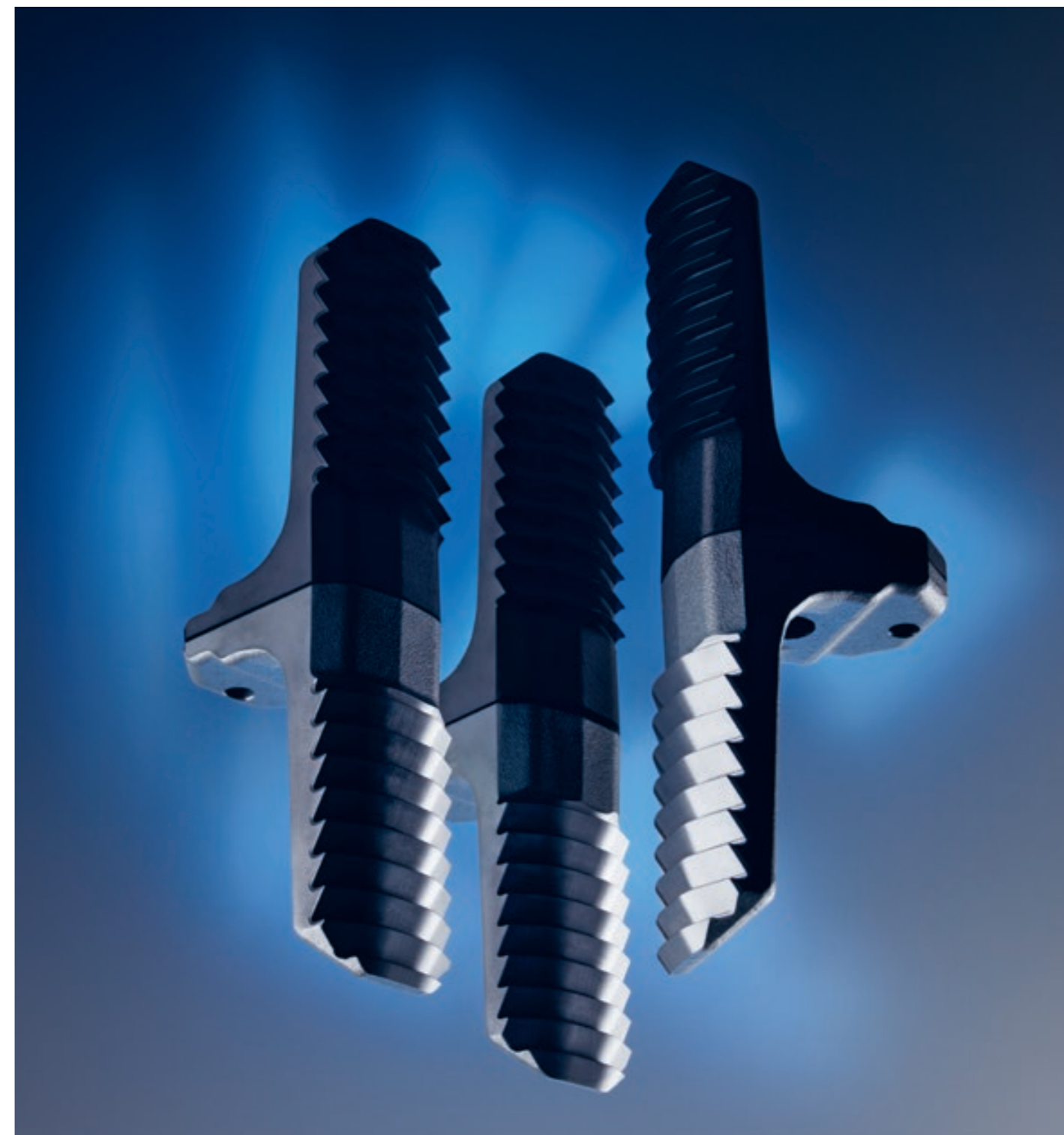
This picture shows a cleaning component of the TruTool TSC 100 slat cleaner in a completely new light. The TruTool removes slag, which accumulates during the cutting process, from the slats of a flatbed laser machine. The two rows of teeth on the cleaning implement clamp onto the slat and slide upwards to scrape off the slag. Photographer Bernd Telle has taken this tool out of its familiar environment and given it a whole new context.
