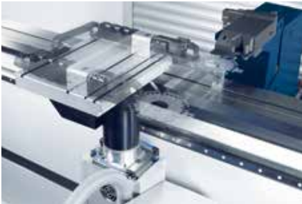
The pivoted-jaw gripper with transversing and rotary axes are highly productive in processing small parts.
