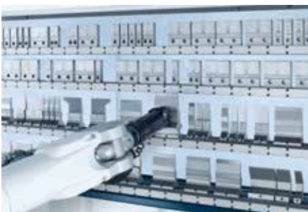
ToolMaster Bend sets up tools completely automatically.
