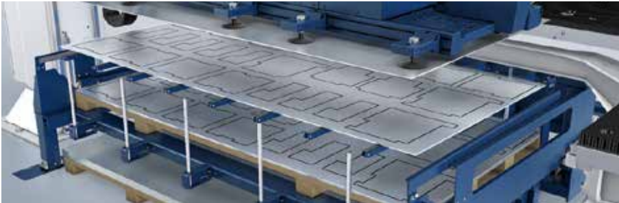
Low-scratch placement of the microjoint sheets with the belt prongs.
