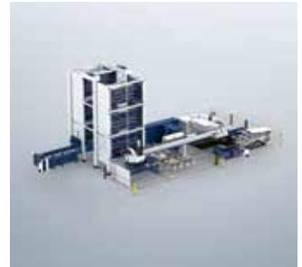
The TruMatic 7000 with SheetMaster and double cart, indirectly connected to the TruStore 3030.
