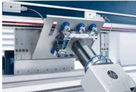
The vacuum gripper for handling large parts.
