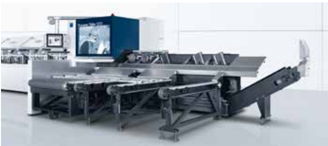
TruLaser Tube 5000 with part removal station and scrap conveyor belt.
